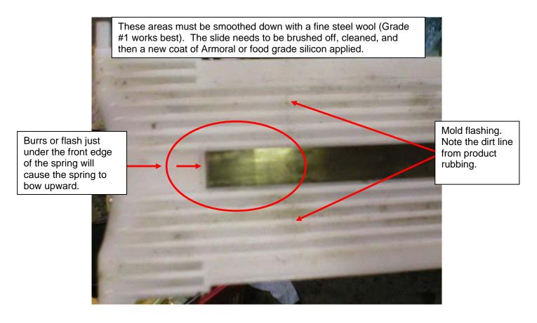
**Issue**: If a Delivery (Picker) Cup plunger trigger is found to have flash or a burr on it where it rides on the cam it may cut in to the cam and slow the push of the target which slows the push of the product in to the cup potentially causing packages to tip and not make it in to the Delivery Cup.
